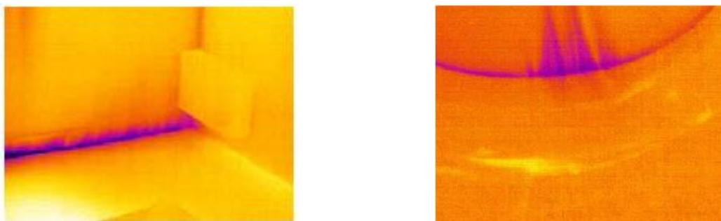
Figure 2: Wall/slabs joints [Cete2006]
