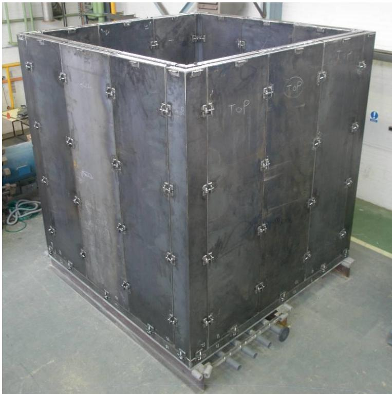
*Figure 22: Picture showing the building physics test facility with the roof removed*
