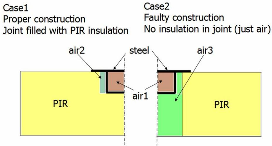
Figure 49: Correct installation of insulation within the joint and compared to missing insulation
