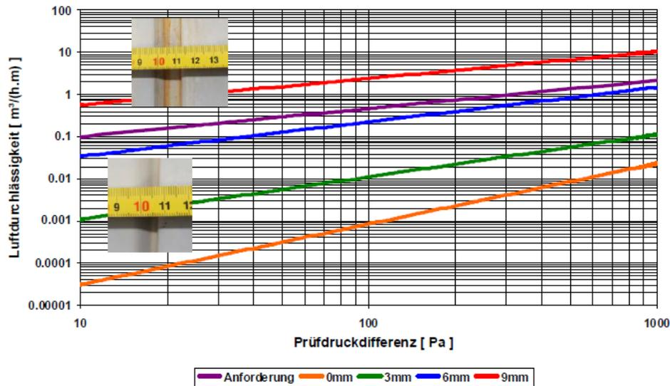
Figure 111: Results for air-tightness of joints (measurements in test rig). Air leakage rate depending of the air pressure difference and several gap widths
