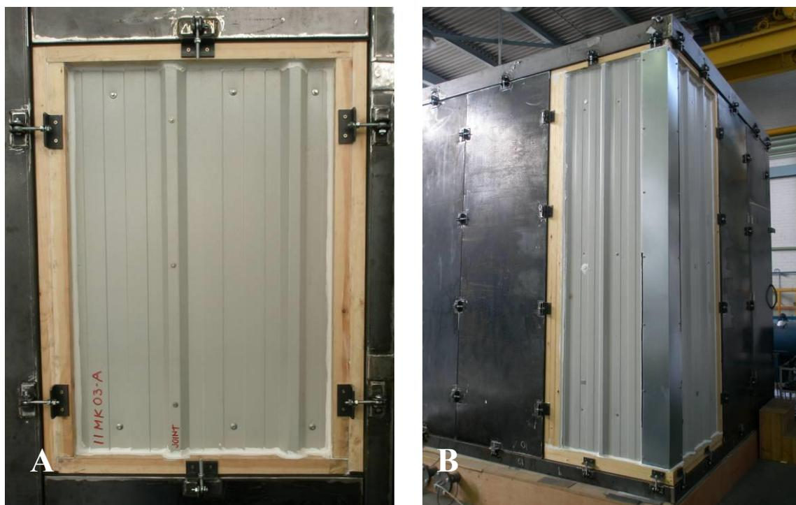
Figure 23: Arrangement of composite panel specimens within test aperture for (A) side and end lap joint tests and (B) external corner joint tests
