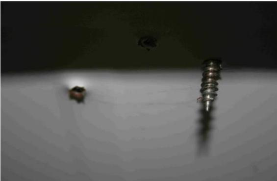
Figure 17: Unused screw punching penetration
