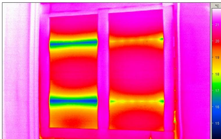
Figure 40: IR-survey (left: conventional cassette, right: thermo-cassette), view from the "hot" side
