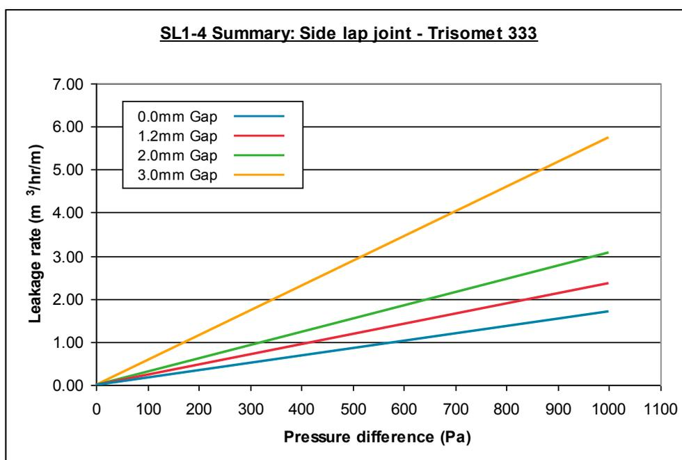
Figure 26: Summary of test results for side lap joint tests SL1 to SL4 – Trisomet 333 composite panel at 0.0 mm, 1.2 mm, 2.0 mm and 3.0 mm joint gaps
