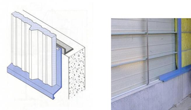
Figure 14: Gap between structural frame and the envelope in this case concrete foundation
