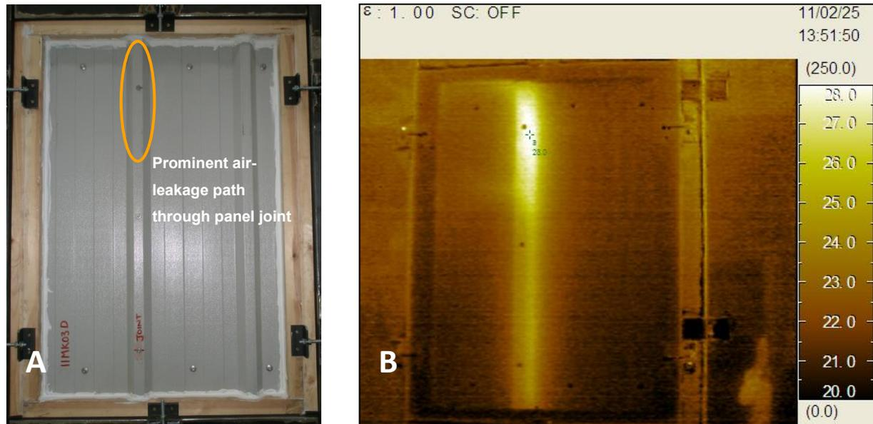
Figure 27: A) Visual image identifying the location of the prominent air leakage path, B) Thermograph taken of the side lap joint test (SL4) at a positive pressure difference of 200 Pa and an internal / external temperature difference of 14 °C
