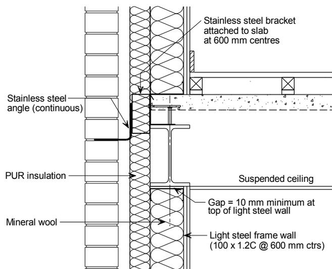
Figure 109: Brickwork attachment to the composite slab
