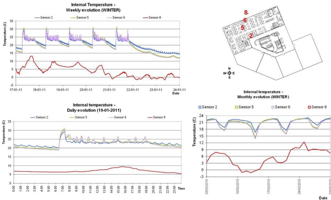
Figure 65: Office building Vitoria, indoor temperatures and monitoring point in the floor plan
