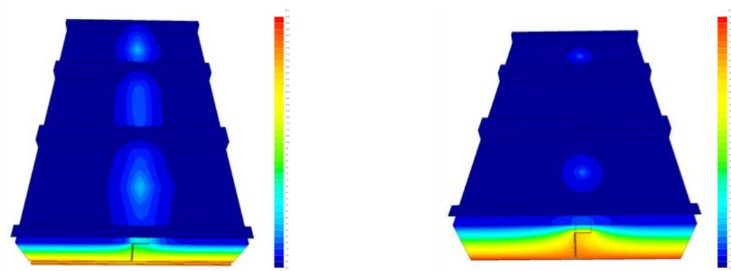
Figure 32: Isotherm within the system without thermal break (left) and with thermal break (right)
