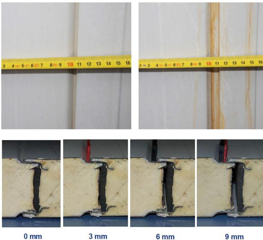
*Figure 110: View of a sandwich wall with various gaps*
