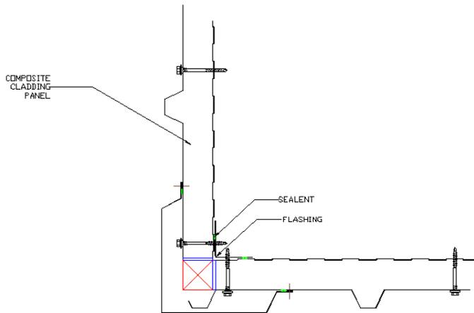
*Figure 112: Example of composite panel system side lap to flashing Joints (as in a vertical corner)*
