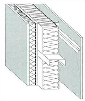
Figure 52: Implementation of a secondary frame
