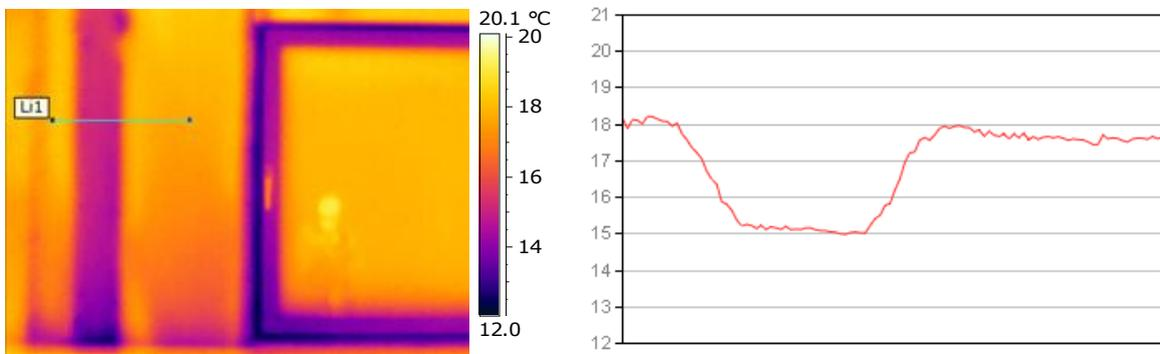
Figure 56: Example of IR survey – Thermal bridge due to a steel beam
