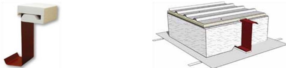
Figure 33: Thermal breaks on Z-girts
