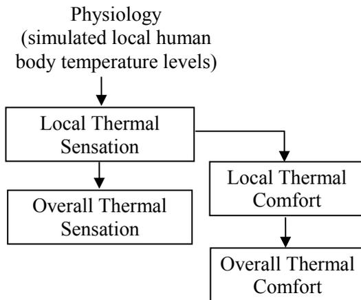
Figure 61: The Overall thermal comfort calculation flow chart
