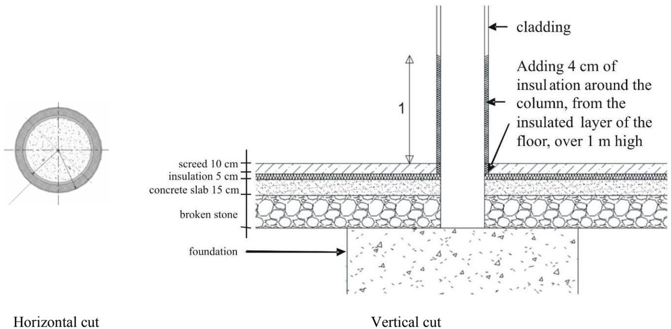
Figure 51: Implementation of thermal break in column/slab interface
