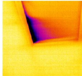
Figure 4: Trough wall openings – Attic access [Cete2006]
