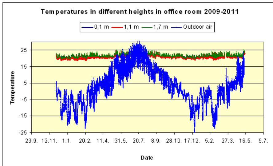
Figure 69: Measured air temperatures in the office room
