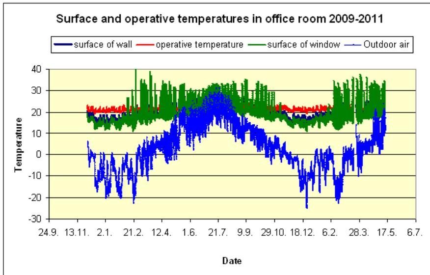
Figure 71: Measured surface and operative temperatures in the office room
