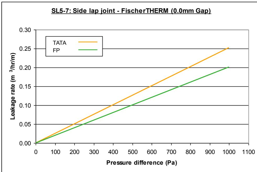
Figure 28: Averaged test results for side lap joint tests SL5 to SL7 – FischerTHERM composite panel at full joint compression compared with previous test results published by Fischer Profil
