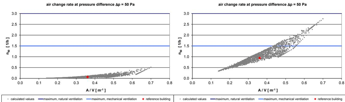
Figure 95: Air-tightness, junctions according class L1 high quality airtight building and class L3 low quality airtight building
