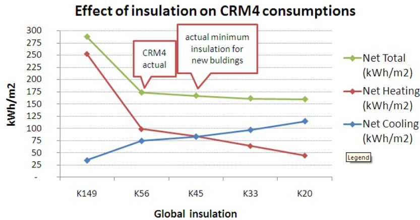
Figure 99: Effect of insulation level on the energy consumption of the building
