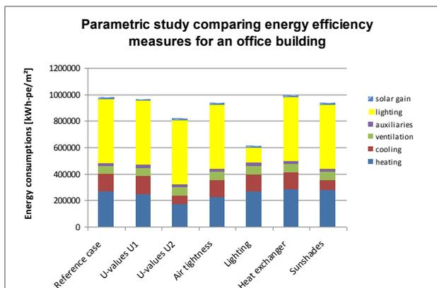
Figure 105: Energy consumption of the Steel Centre building with various measures
