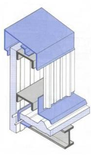
Figure 16: Air gaps in acroterium arrangement
