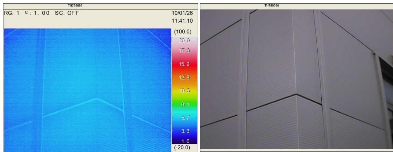
Figure 47: A planar composite panel corner junction performing as intended
