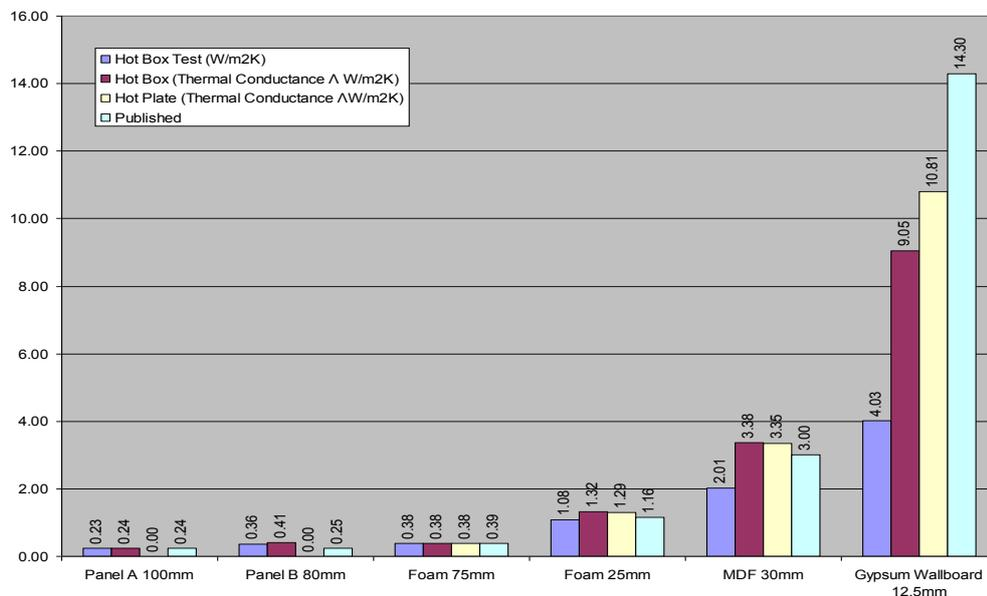
Figure 38: Results obtained from guarded hot box, hot plate and published sources
