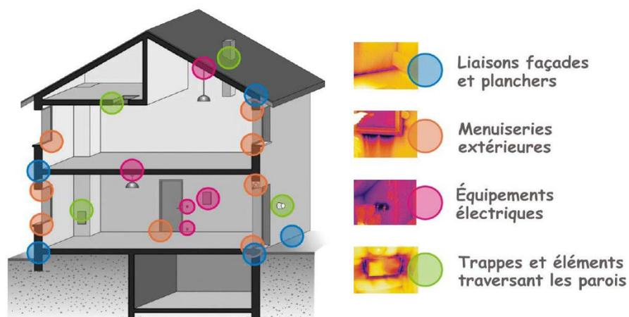
Figure 1: Example of typical air gaps [Cete2006]
