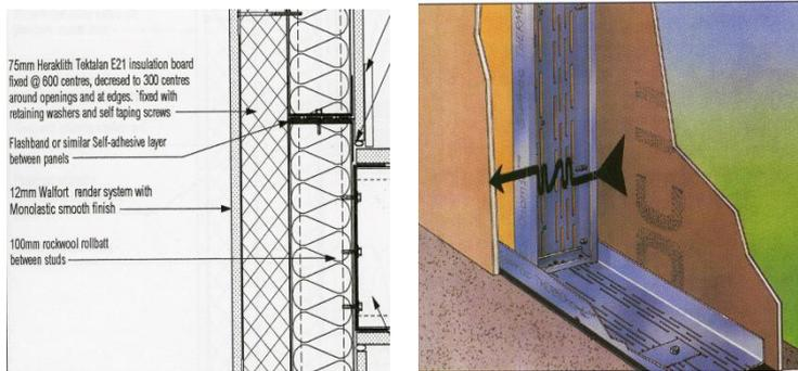
Figure 107: Wall section illustrating the warm frame, solid-wall construction with slotted steel studs
