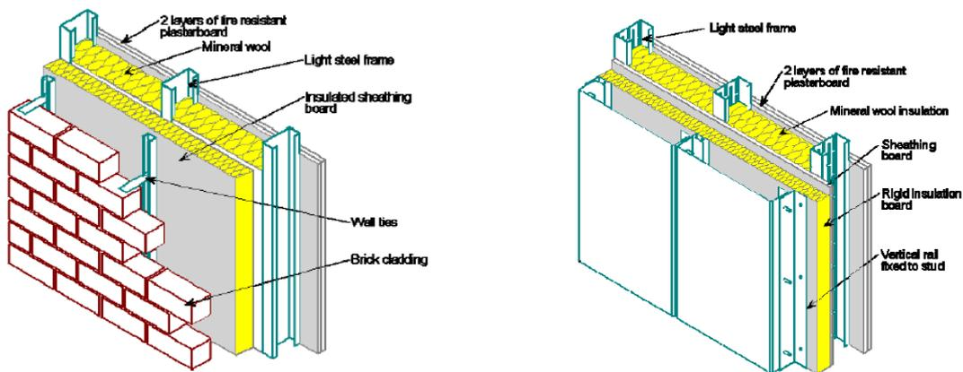
Figure 108: Ventilated facade systems using two types of cladding [SCI]
