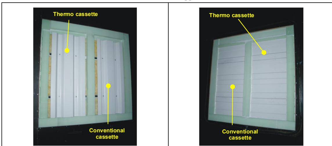
Figure 39: Cassette wall systems in hot-box (left: view "cold" side, right: view "hot" side)
