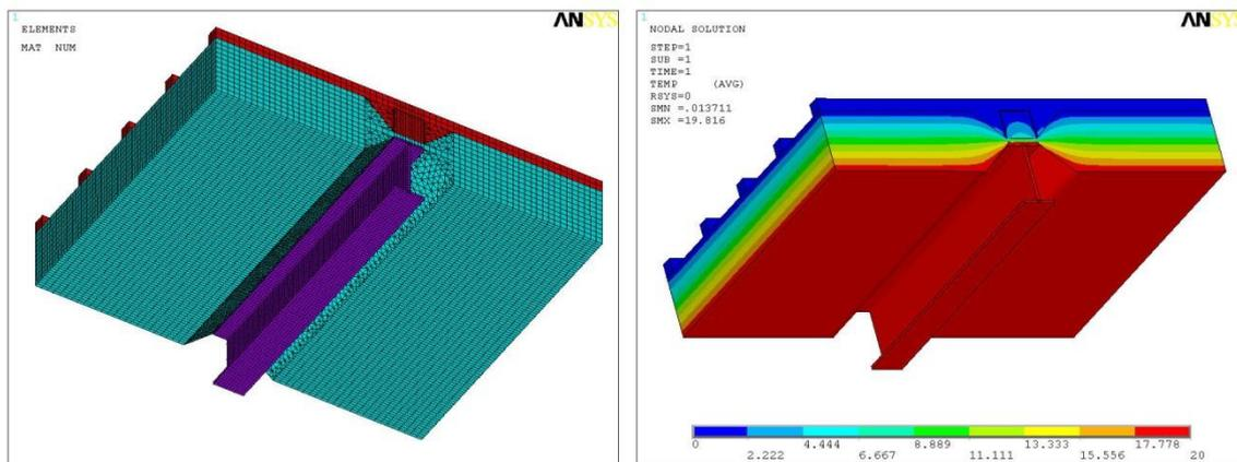
Figure 55: Example of FE calculation of 2D thermal bridge
