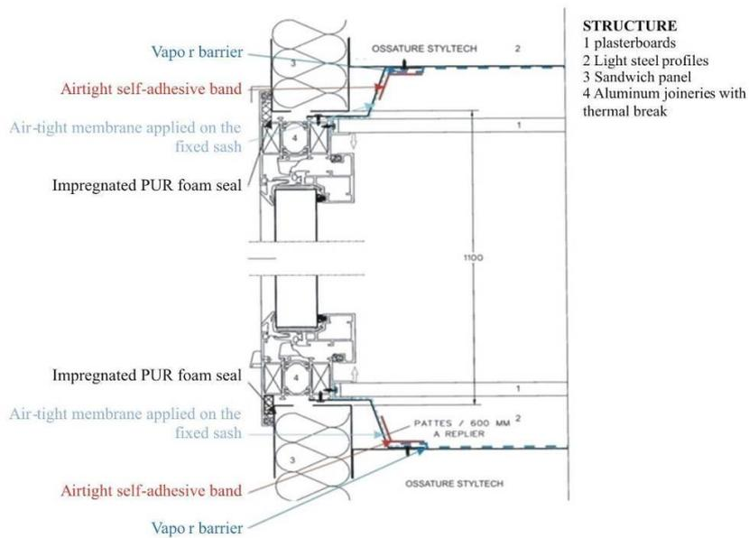
Figure 50: Vertical cut within a window displaying a good practice to improve the air-tightness of the joineries
