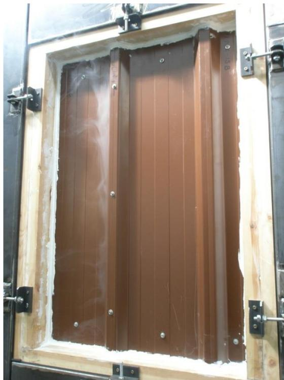
Figure 29: Leakage through the side lap joint test of the FischerTHERM composite panel at an internal pressure difference of 600 Pa, confirmed using smoke testing
