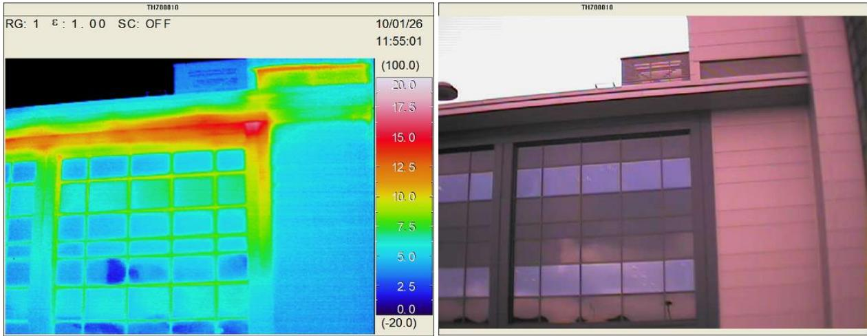
Figure 41: Thermal image showing an intense accumulation of internal hot air at the corner of the built-up architectural feature, as indicated by the red contours. Measurements show a temperature difference of +10 °C between the built-up feature and the adjacent composite panels
