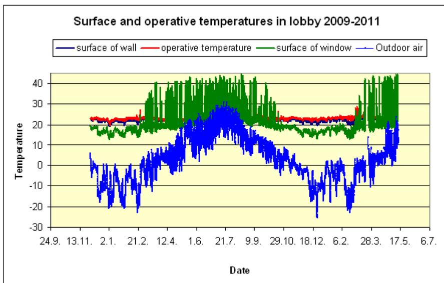
Figure 72: Measured surface and operative temperatures in the lobby
